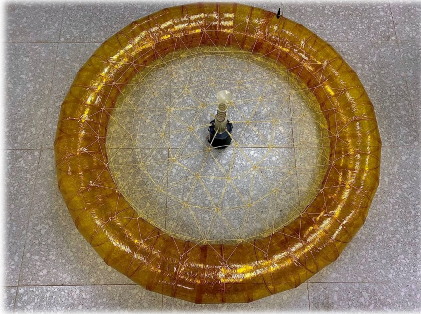
Figure 8. The completed inflatable cable net antenna principle prototype with a diameter of 1.4m.
