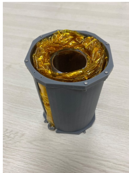
Figure 9. The main reflector can be fitted in 1.5U ( 10 \times 10 \times 15 \text{cm}^3 ) even when it is not fully evacuated.
